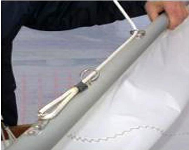
**d) After hoisting, the surplus sail can be kept tidy by tying up the three reefing lines round the boom.**
