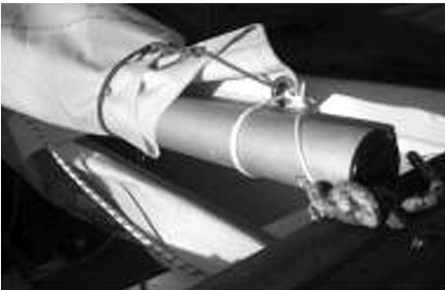
b) Pass the leech reefing line through the clew cringle and back through the leech cringle, tension it and tie off round the boom. This will hold the reef down and flatten the sale.
