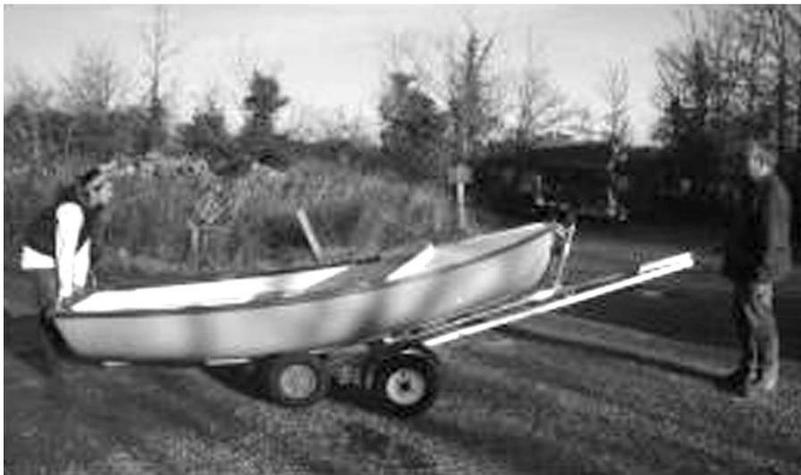
Release downward pressure on the transom, then use foot to press down on the tow bar and the launch trolley will slide forward. Secure trolley to trailer with drop-nose pins.
