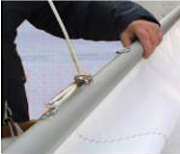
**c) After hoisting the mainsail and tensioning the downhaul, there should be a 3" (75 mm) gap between the gaff and the main halyard mast block. This allows for articulation and avoids block damage.**
