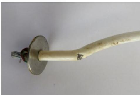
How does this happen? Interestingly every time you put the cover on you bend the stop and over time the stainless steel wire is work hardened and becomes brittle, ultimately breaking. The more you sail the more likely the damage
